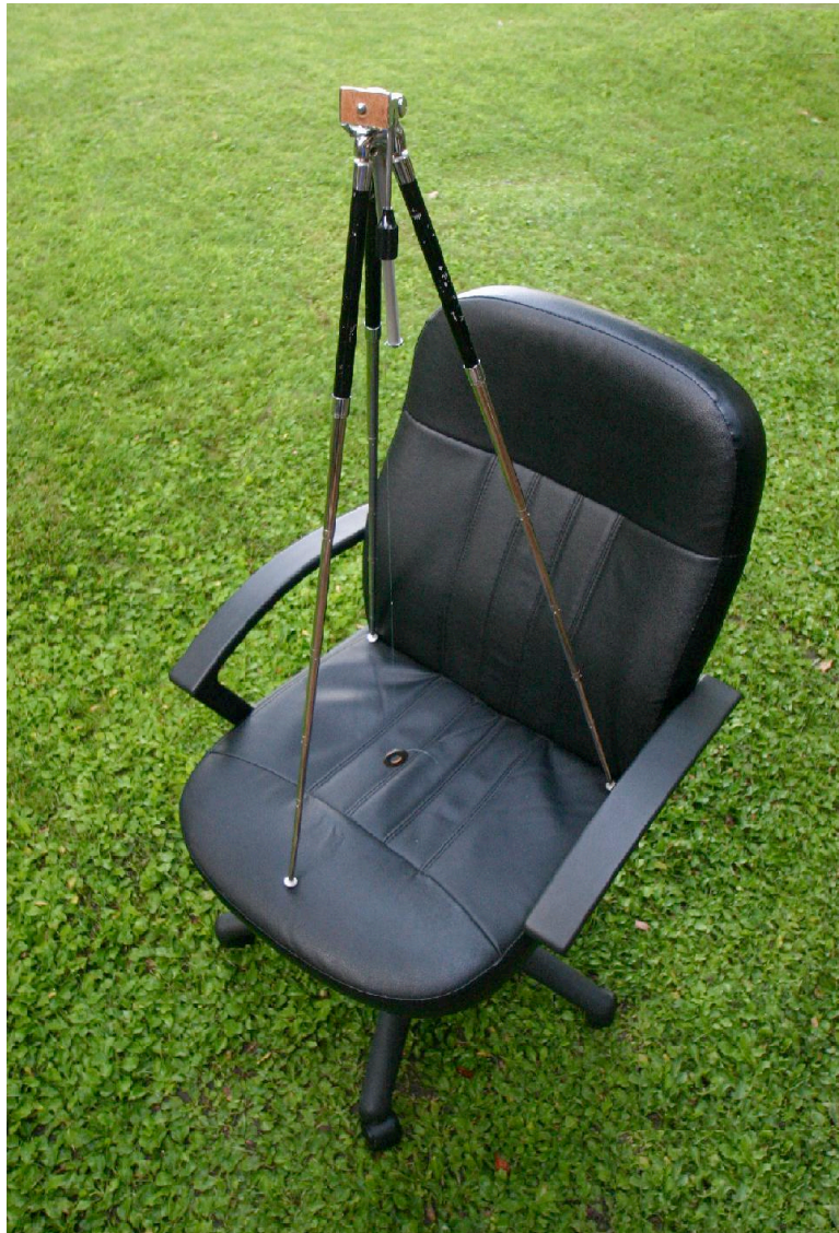
Figure 1. A rickety old tripod is entirely adequate for this demonstration. The pendulum bob, a large washer, hangs from the bottom of center post.
