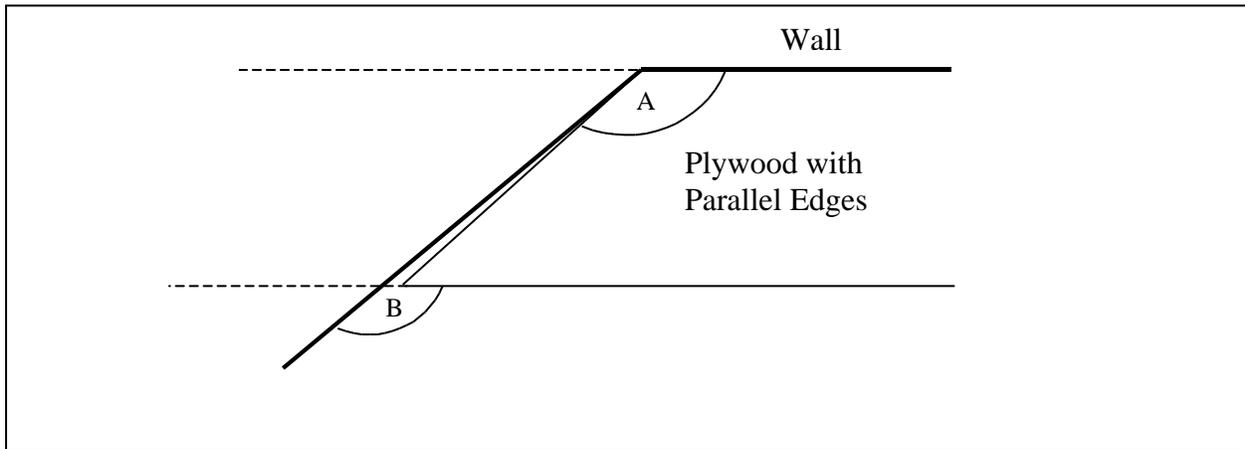
We want to measure the angle between the two walls, A. Using the fact that the two edges of the plywood are parallel, we can use congruent angles to measure the angle B where the plywood meets the straight wall and we will know the angle we need!
