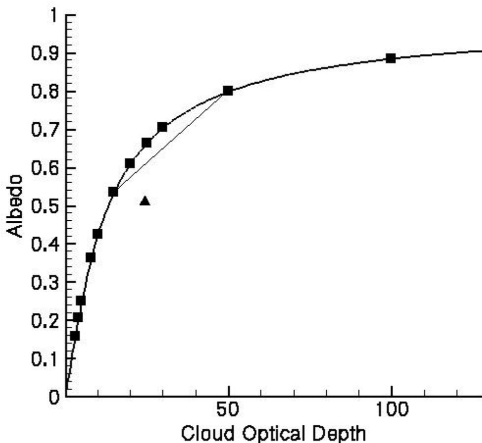
Figure 1. Albedo versus cloud optical depth, a nonlinear phenomenon.
